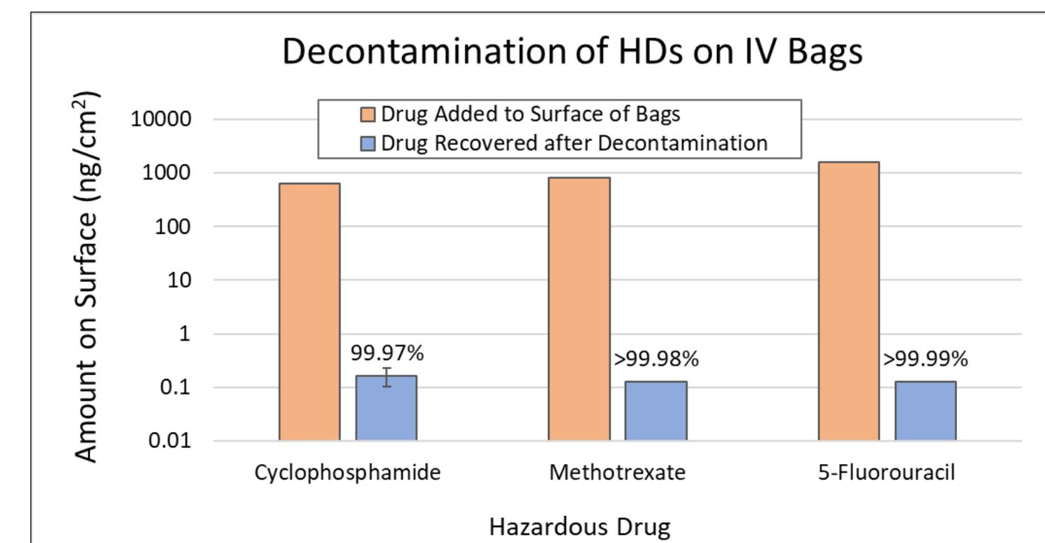
**Results:** The EPA-registered one-step disinfectant effectively decontaminated multiple HDs from the IV bags.
